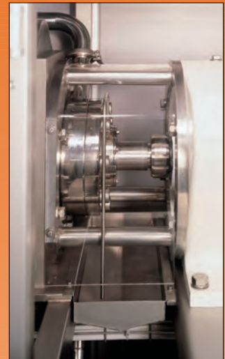
Hot water seal flushing as standard
